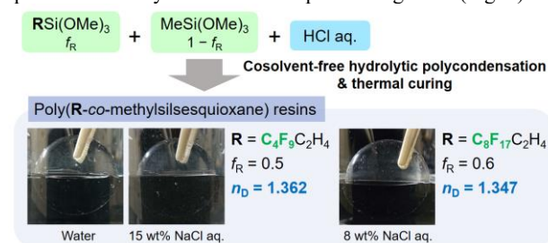
Fig. 3 Fluorine-containing low-refractive-index polysilsesquioxane resins prepared by a cosolvent-free method.
