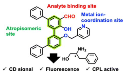
Figure 5. Chiral recognition using quaterphenyl-5'-carbaldehyde.
